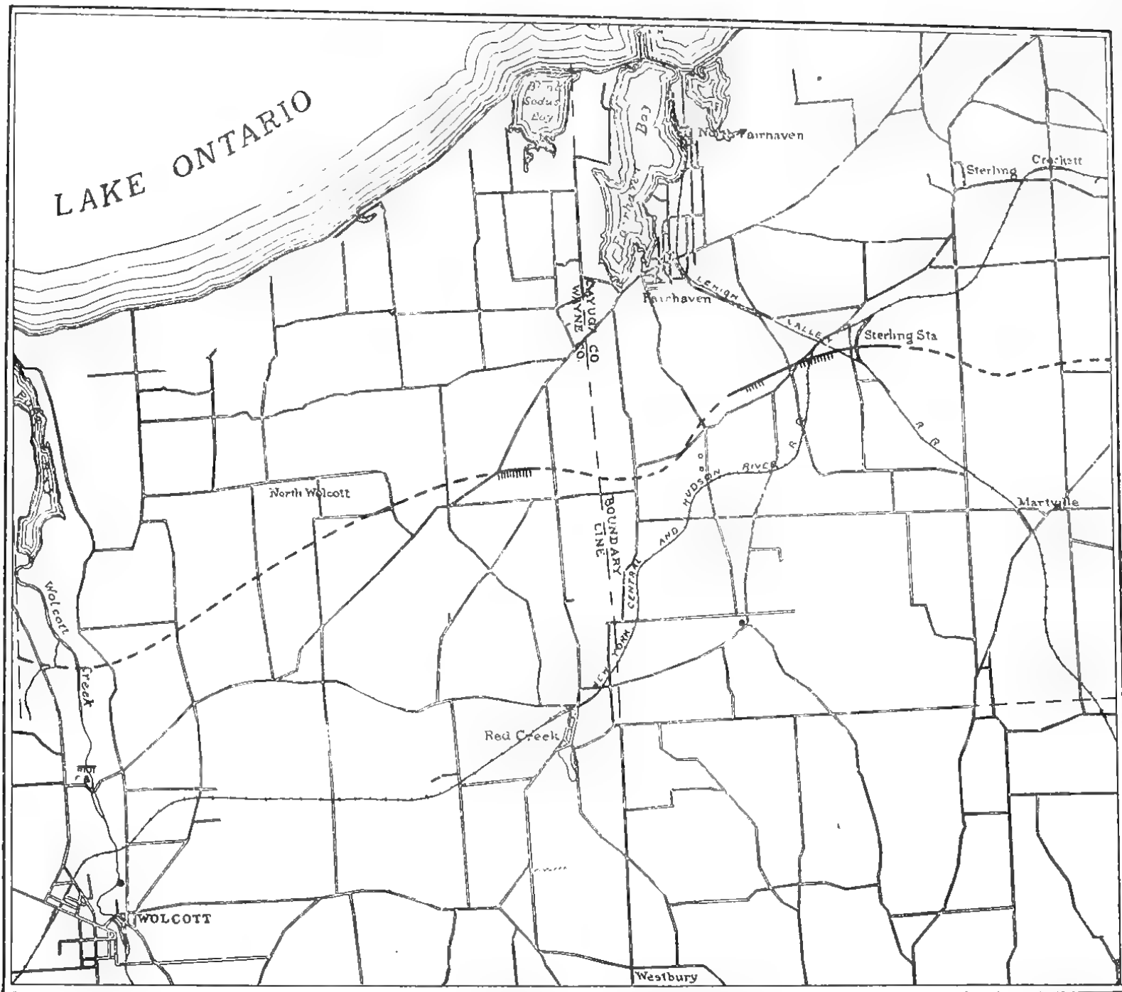
Fig. 3 Sketch map of the Clinton ore belt in Cayuga and eastern Wayne counties. The approximate outcrop of the lower or main ore bed is indicated by the broken line. The map also shows the outcrop of the upper ore seam north of Wolcott and position of the recent test holes. Scale 1 mile to \frac{1}{2} inch
